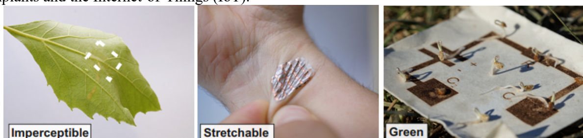
Figure. Flexible Electronics with different functionalities (from left to right): transparency, mechanical flexibility and biocompatibility.
